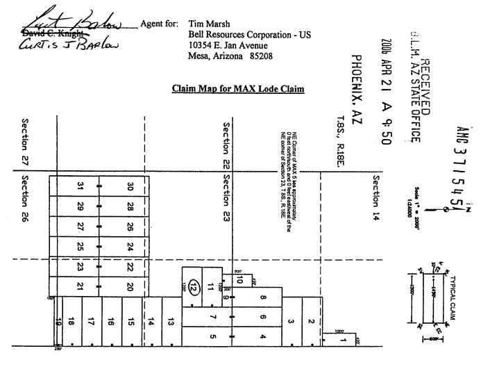
The above map depicts the MAX 12 lode mining claim, which is located in Section (s) 23, Township 8 South, Range 18 East, Gila and Salt River Base Meridian, Pinal County, Arizona. The claim corners, end centers, and location monument are marked by 2 inch by 2 inch by 5 foot wooden posts with aluminum tags. The bearings and distances between claim corners are as depicted on the map.
