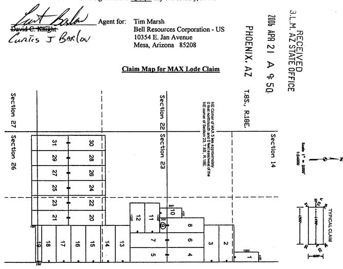
The above map depicts the  $MAX \underline{9}$  lode mining claim, which is located in Section (s)  $\underline{23}$ , Township 8 South, Range 18 East, Gila and Salt River Base Meridian, Pinal County, Arizona. The claim corners, end centers, and location monument are marked by 2 inch by 2 inch by 5 foot wooden posts with aluminum tags. The bearings and distances between claim corners are as depicted on the map.
