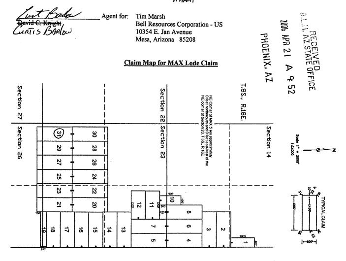
The above map depicts the MAX 3/ lode mining claim, which is located in Section (s) 23 426, Township 8 South, Range 18 East, Gila and Salt River Base Meridian, Pinal County, Arizona. The claim corners, end centers, and location monument are marked by 2 inch by 2 inch by 5 foot wooden posts with aluminum tags. The bearings and distances between claim corners are as depicted on the map.
