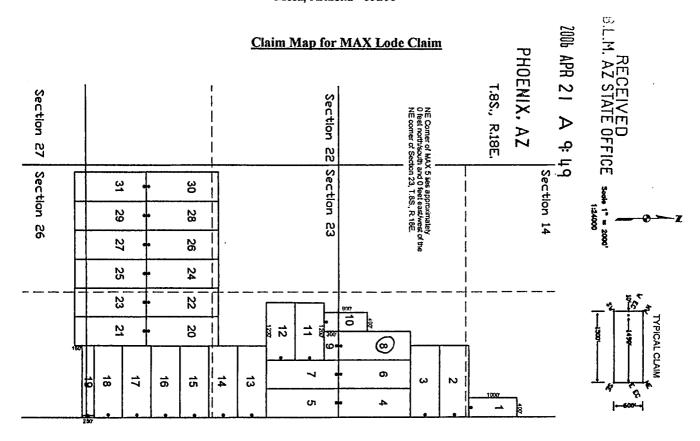
The above map depicts the MAX 8 lode mining claim, which is located in Section (s) 148 South, Range 18 East, Gila and Salt River Base Meridian, Pinal County, Arizona. The claim corners, end centers, and location monument are marked by 2 inch by 2 inch by 5 foot wooden posts with aluminum tags. The bearings and distances between claim corners are as depicted on the map.
