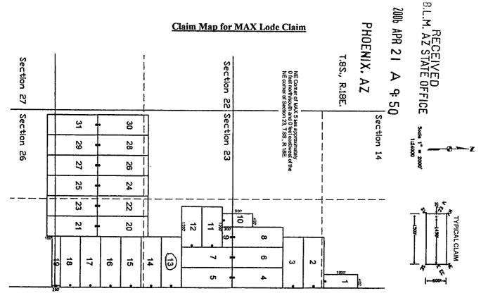
The above map depicts the MAX 13 lode mining claim, which is located in Section (s) 238 South, Range 18 East, Gila and Salt River Base Meridian, Pinal County, Arizona. The claim corners, end centers, and location monument are marked by 2 inch by 2 inch by 5 foot wooden posts with aluminum tags. The bearings and distances between claim corners are as depicted on the map.
