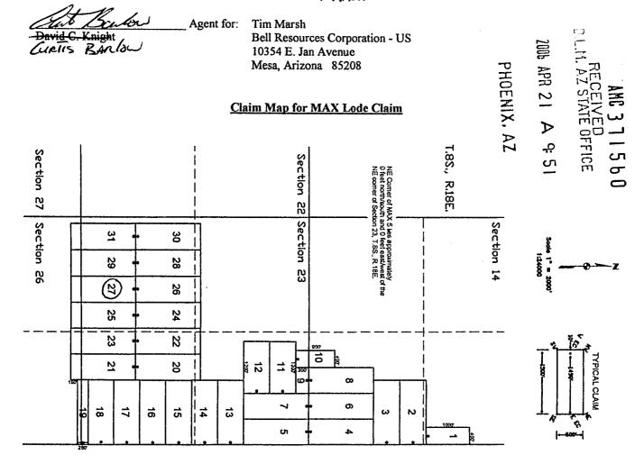
The above map depicts the MAX Z7 lode mining claim, which is located in Section (s) 23 126. Township 8 South, Range 18 East, Gila and Salt River Base Meridian, Pinal County, Arizona. The claim corners, end centers, and location monument are marked by 2 inch by 2 inch by 5 foot wooden posts with aluminum tags. The bearings and distances between claim corners are as depicted on the map.
