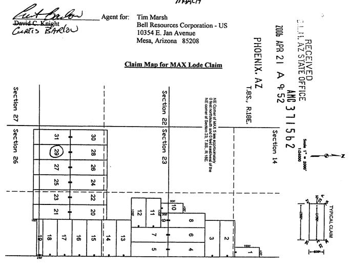
The above map depicts the MAX 29 lode mining claim, which is located in Section (s) 23 426, Township 8 South, Range 18 East, Gila and Salt River Base Meridian, Pinal County, Arizona. The claim corners, end centers, and location monument are marked by 2 inch by 2 inch by 5 foot wooden posts with aluminum tags. The bearings and distances between claim corners are as depicted on the map.
