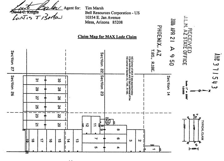
The above map depicts the MAX 10 lode mining claim, which is located in Section (s) 14+23, Township 8 South, Range 18 East, Gila and Salt River Base Meridian, Pinal County, Arizona. The claim corners, end centers, and location monument are marked by 2 inch by 2 inch by 5 foot wooden posts with aluminum tags. The bearings and distances between claim corners are as depicted on the map.
